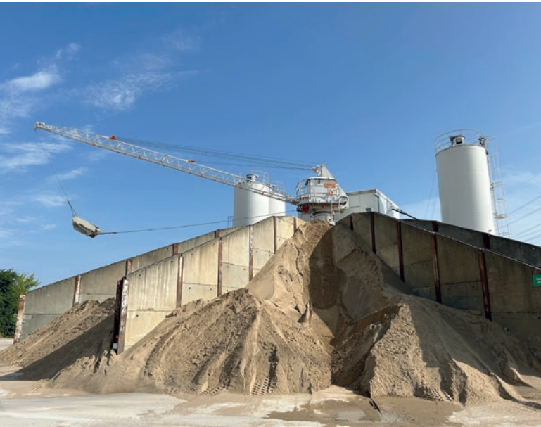
The scope of the modernisation also includes a THS 60/20 automatic scraper with a 22 m boom.
