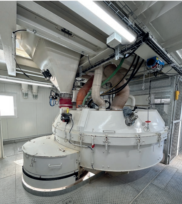
The centrepiece of the new concrete mixing plant is the THZ 3000 turbine mixer from Teka.
