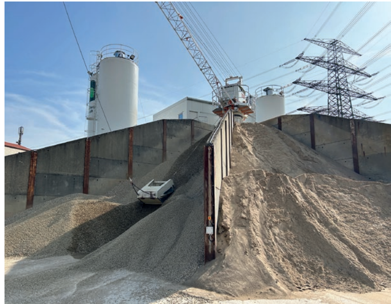
The scope of the modernisation also includes a THS 60/20 automatic scraper with a 22 m boom.
