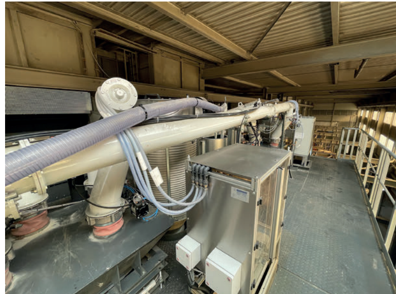
Teka's scope of supply also included a weighing platform, storage containers for the aggregates, binding agent scales, dedusting filter units, binding agent screws and a fibre dosing system.
