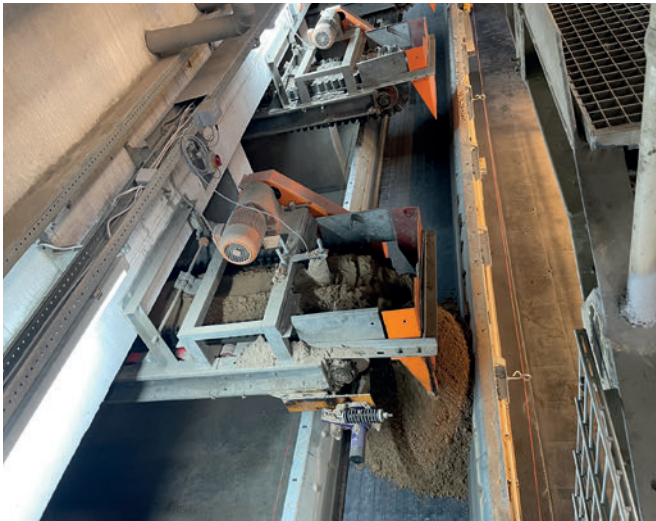
The flat design of the weigh belts is ideally adapted to the available space.
