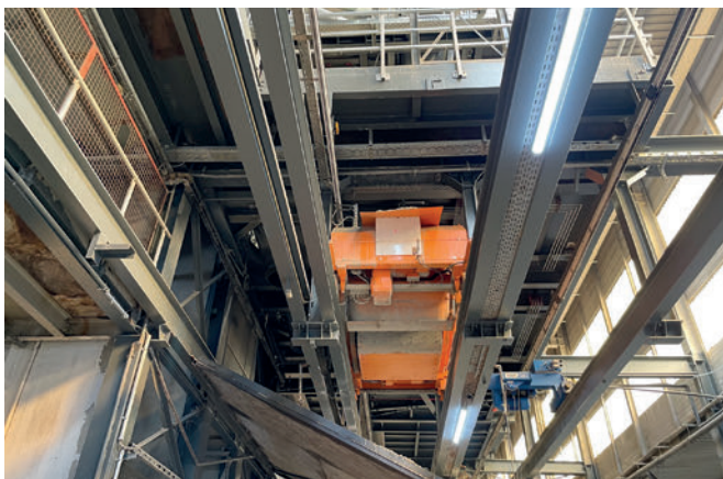
Two Kübat bucket conveyors ensure concrete transport in production
