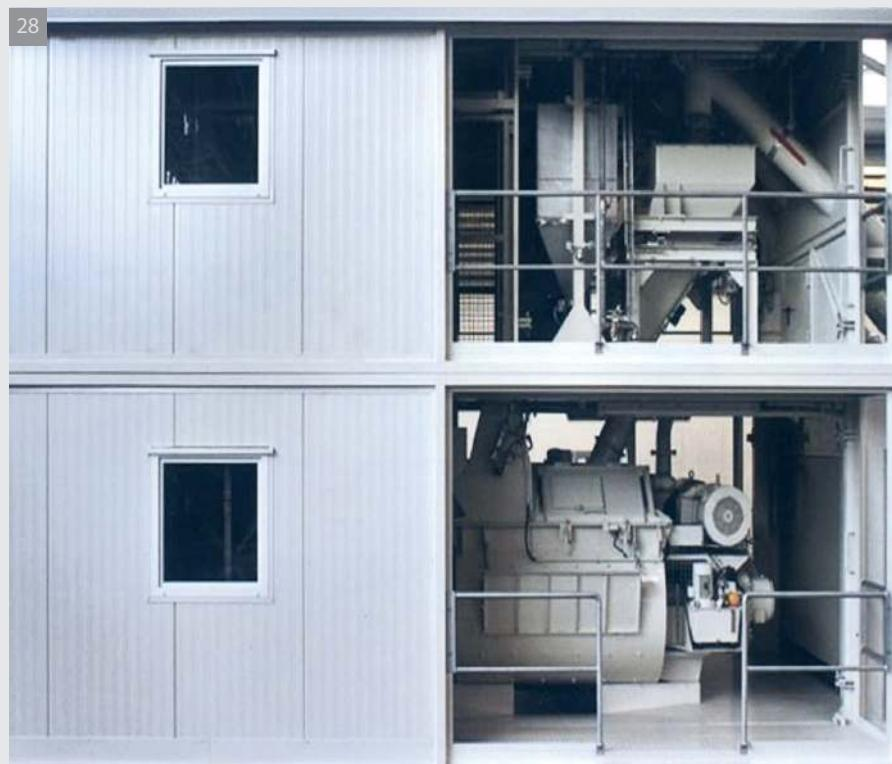
28-31 | The MIXOMAT D is a fast erection concrete mixing plant with an aggregate in-line silo system for feeding of aggregates by means of a shovel-loader. Completely pre-assembled modules allow for very quick set-up times for erection and disassembly. Maximum transportation width of the mixing plant is 3,0 meters.
