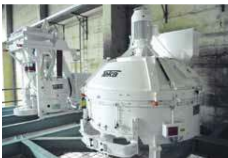
Modification with high-performance Teka turbine mixer THT 250 and THT 1125 for the production of face mix concrete and core concrete
