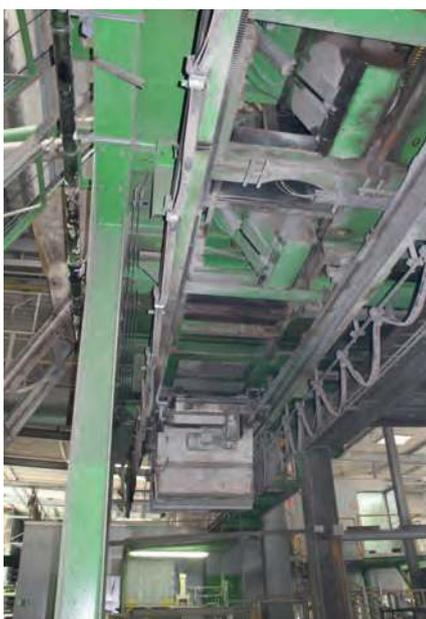
Like the core concrete mixers, the new high performance turbine mixers discharge directly into one of the two flying buckets.
