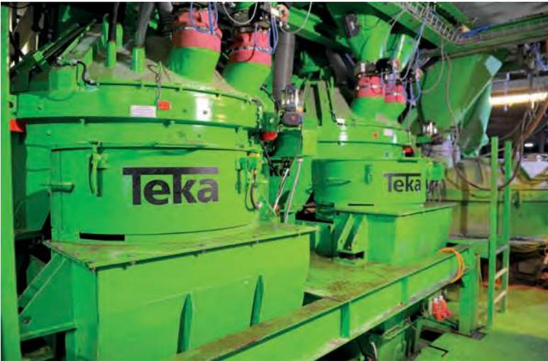
The two Teka THT E-1-III high performance turbine mixers for high-quality facing concretes.
