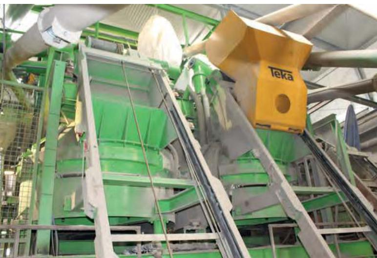
Teka installed two skip hoists (500 litres) in a bottom discharge design to complement the two new facing concrete mixers.
