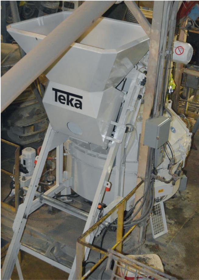
*The Teka Skip Hoist has a bottom-discharge bucket, and travels on the 60° angle track, quickly delivering batch materials to the mixer, which is over 25' above the plant floor.*
