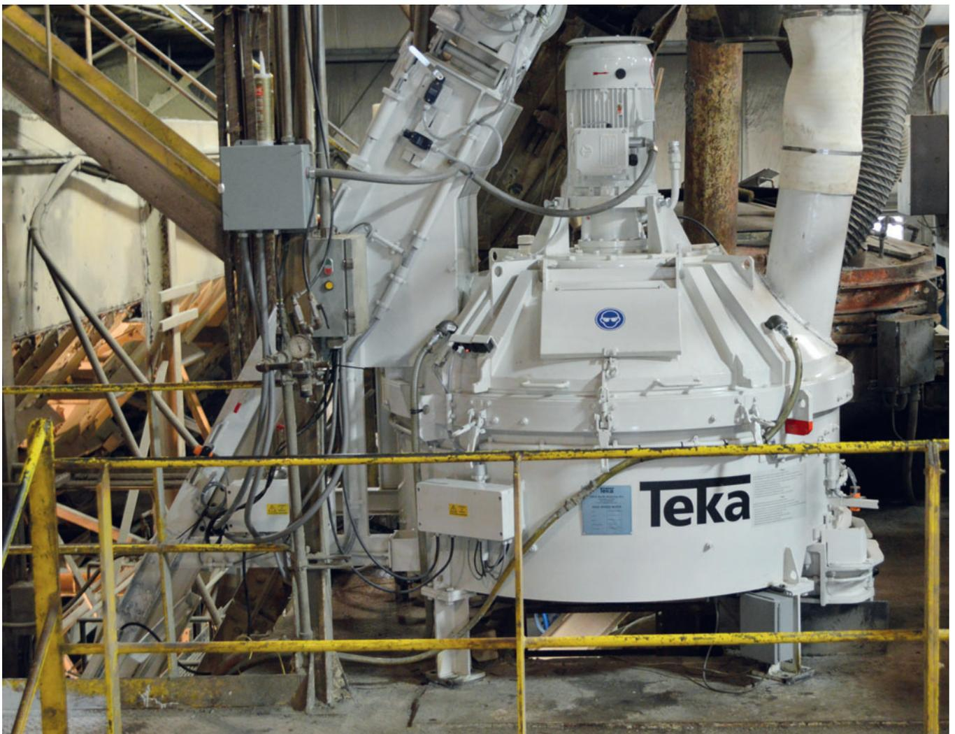
*Doren, Inc. chose the Teka THT 500 C-1-II mixer model with a Teka Skip Hoist. Like all THT mixers, it comes standard with a Variable Frequency Drive that allows producers to choose mixer speeds that best suit specific mix designs.*
