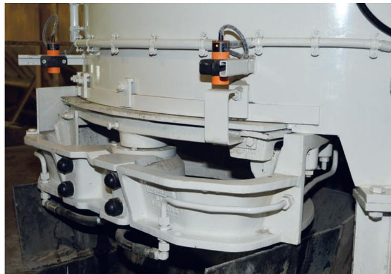
*Teka discharge gates are operated by a powerful hydraulic rotary cylinder. If needed, multiple proximity switches can be added to allow for partial openings of the gate.*
