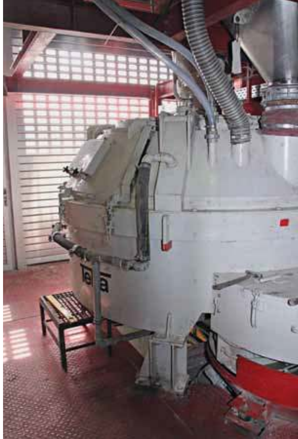
One of the two identical Teka turbine mixers on the new platform
