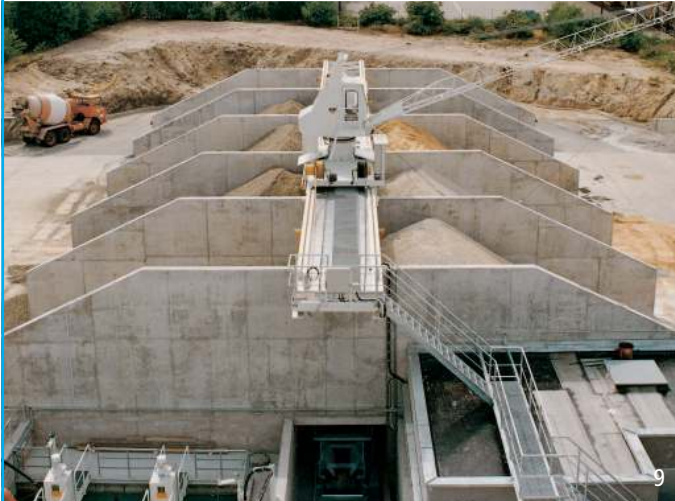
Picture 8 & 9: Compact Batching and Mixing Plant MIXOMAT THZ 3000 B2-R8, with fully automatic Heavy Duty Scraper THS 40/16, in linear operation.
