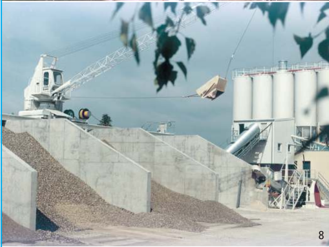
Picture 5: Compact Batching and Mixing Plant MIXOMAT THZ 3000 B1-S5 with fully automatic Heavy Duty Scraper THS 60/22.
