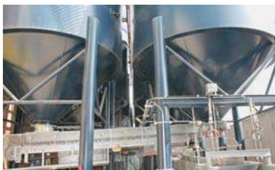
**Fig. 3** The aggregates are transported from the new silos to the concrete mixing tower by weigh belts.
