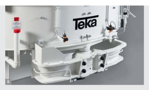
use the same oil for less maintenance. This oil also supplies the pressure to operate the discharge gate(s).
