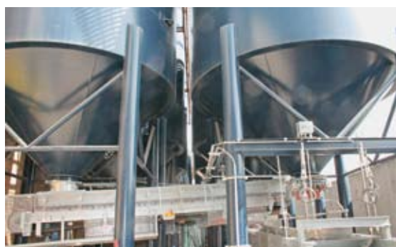
Fig. 3 The aggregates are transported from the new silos to the concrete mixing tower by weigh belts.
